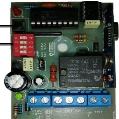
EXTERNAL CABLED RECEIVER
