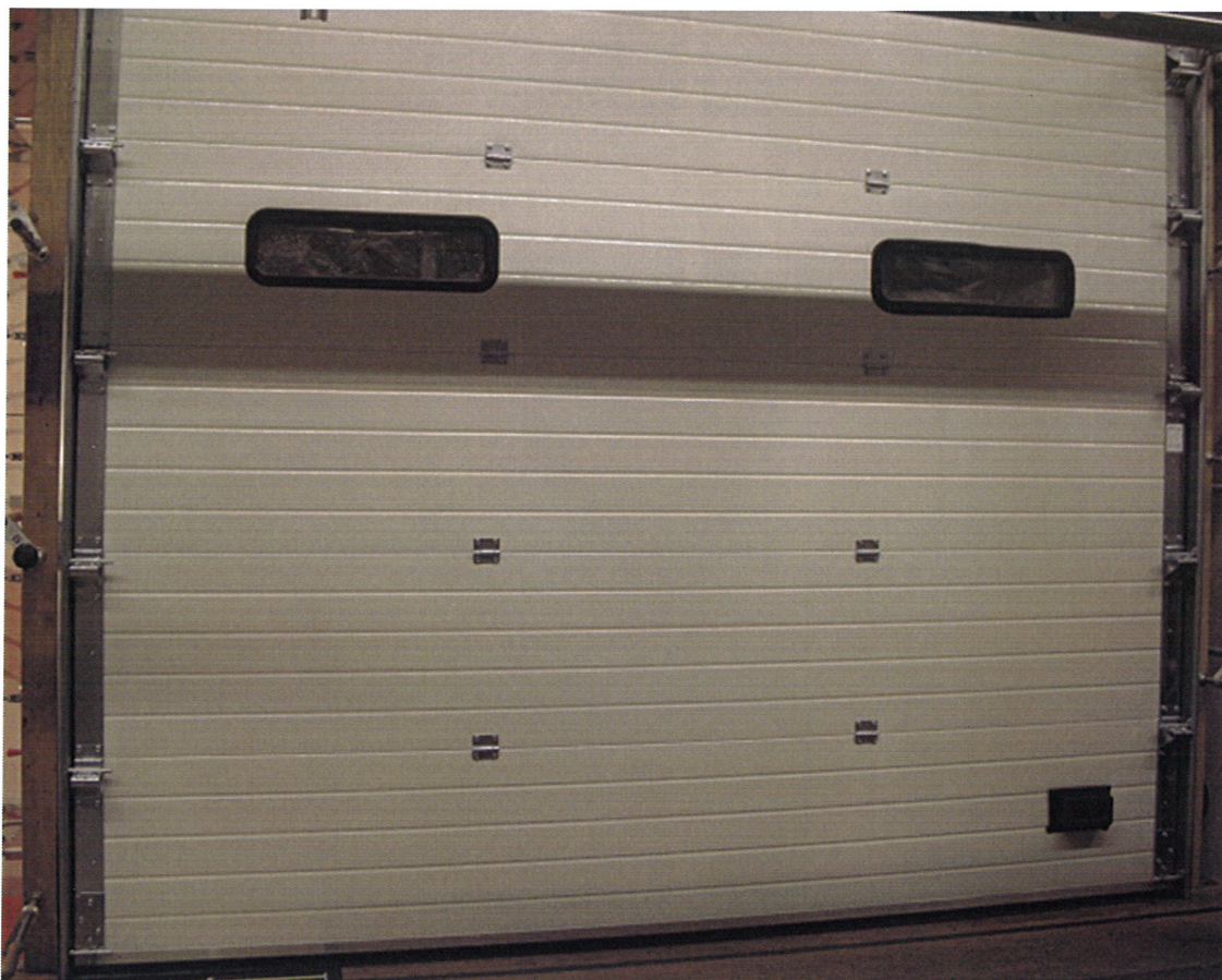
Figure 2. Door type Alkur Normtor, mounted in the test rig, as seen from inside.
