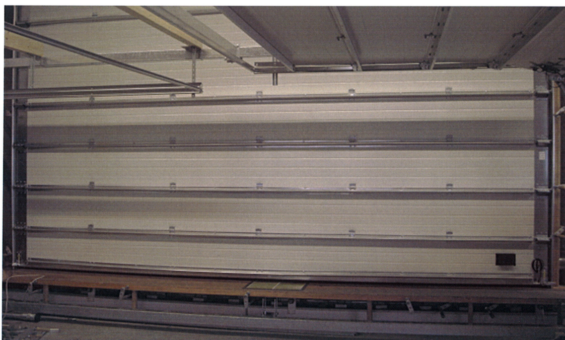
Figure 2. Door type Alkur Normtor, mounted in the test rig, as seen from inside.
